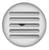
The interior temperature sensor, located on the instrument panel to the right of the steering wheel, measures the temperature of the air inside the vehicle.
